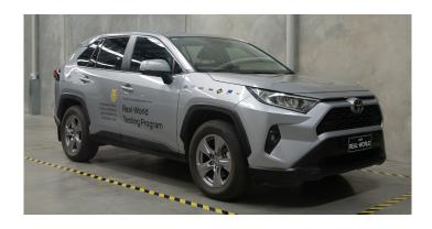
The Real-World Testing Program tested a 2022 Toyota RAV4 with a 2.0 litre petrol engine. In the real-world tests, per kilometre the RAV4 used 13% more fuel than the mandated lab test and emitted 13% more CO<sub>2</sub> emissions.
