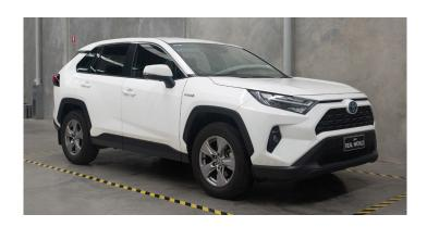
The Real-World Testing Program tested a 2022 Toyota RAV4 with a 2.5 litre hybrid petrol/electric engine. In the real-world tests, per kilometre the RAV4 used 2% more fuel than the mandated lab test and emitted 3% more CO<sub>2</sub> emissions.
