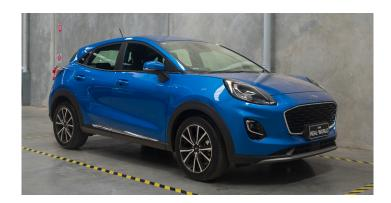
The Real-World Testing Program tested a 2022 Ford Puma with a 1.0 litre turbo petrol engine. In the realworld tests, per kilometre the Puma used 8% more fuel than the mandated lab test and emitted 10% more CO<sub>2</sub> emissions.
